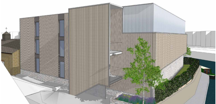
Indicative bird's eye view of the northern elevation showing the staircase enclosure and window details
